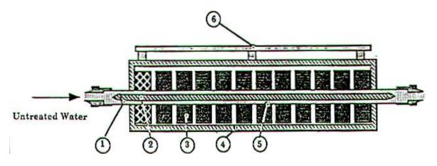
Fig. 2 Electromagnetic Device for Magnetic Treatment of Water.
